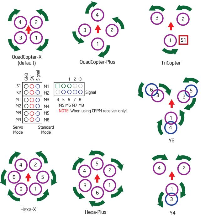
NOTE In Tri-Copter mode, tail tilt servo connects to S1, and motors M1..M3 as shown on the diagram above. When camera stabilization is enabled, gimbal pitch/roll servos connect to S1/S2, and motor connectors shift as well.
