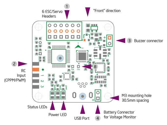
Board is 36x36mm square, with mounting holes for M3 screws, spaced 30.5mm.
