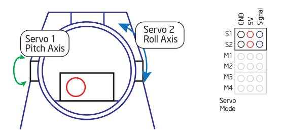
WARNING If using high-current-draw servos for camera stabilization, consider powering them from a separate BEC. Only connect Signal and GND wire to the board, and 5V wire from servos to a separate power source.
